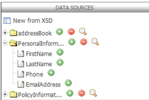
To generate a group control that automatically includes controls for all of a parent element's children, click the icon to the right of the complex type's folder icon. The controls for the children elements will be inside a section control. If the complex type has repeating items, the section will be inside a repeat control.
